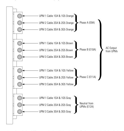
**NOTE** Two cable lugs will be connected to each terminal stud. When connecting the cable lugs, install the first lug on the stud with the raised barrel portion facing the back of the cabinet. Install the second lug with the raised barrel portion facing the front of the cabinet.
